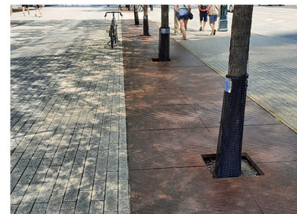
Trees in hard paving with connected soil volumes
